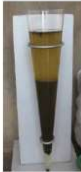
Imhoff Cone with settleable solids
